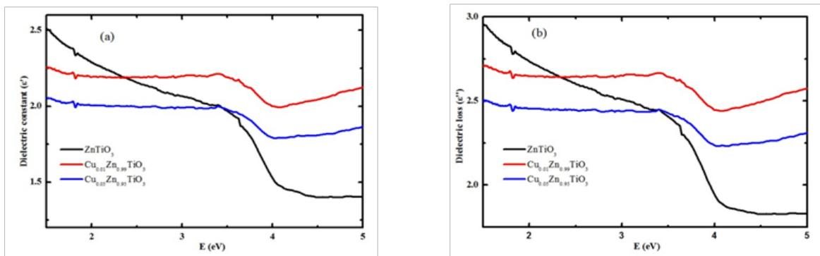
Fig. 6. (a) Real part, (b) Imaginary part of dielectric constant as a function of photon energy for ZnTiO<sub>3</sub>, Cu<sub>0.01</sub>Zn<sub>0.99</sub>TiO<sub>3</sub> and Cu<sub>0.05</sub>Zn<sub>0.95</sub>TiO<sub>3</sub> thin films.
