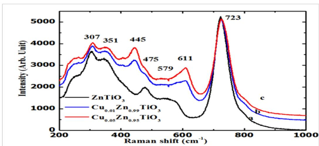
Fig. 2. Raman shift of thin films (a)  $\text{ZnTiO}_3$  doped with two different concentrations of Cu ions (b) 1 and (c) 5 mol% deposited on quartz substrates and annealed at 600 °C for 1 h.
