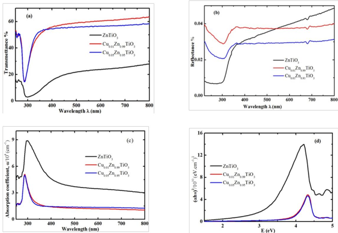
Fig. 4. (a) Transmittance, (b) Reflectance, and (c) Absorption coefficient as functions of wavelength. (d)  $(ah\nu)^2$  as a function of photon energy for  $\text{ZnTiO}_3$ ,  $\text{Zn}_{0.99}\text{Cu}_{0.01}\text{TiO}_3$  and  $\text{Zn}_{0.95}\text{Cu}_{0.05}\text{TiO}_3$  thin films with thickness 250, 276 and 300 nm, respectively, deposited on glass substrates and annealed at  $400^\circ\text{C}$  for 1 h.
