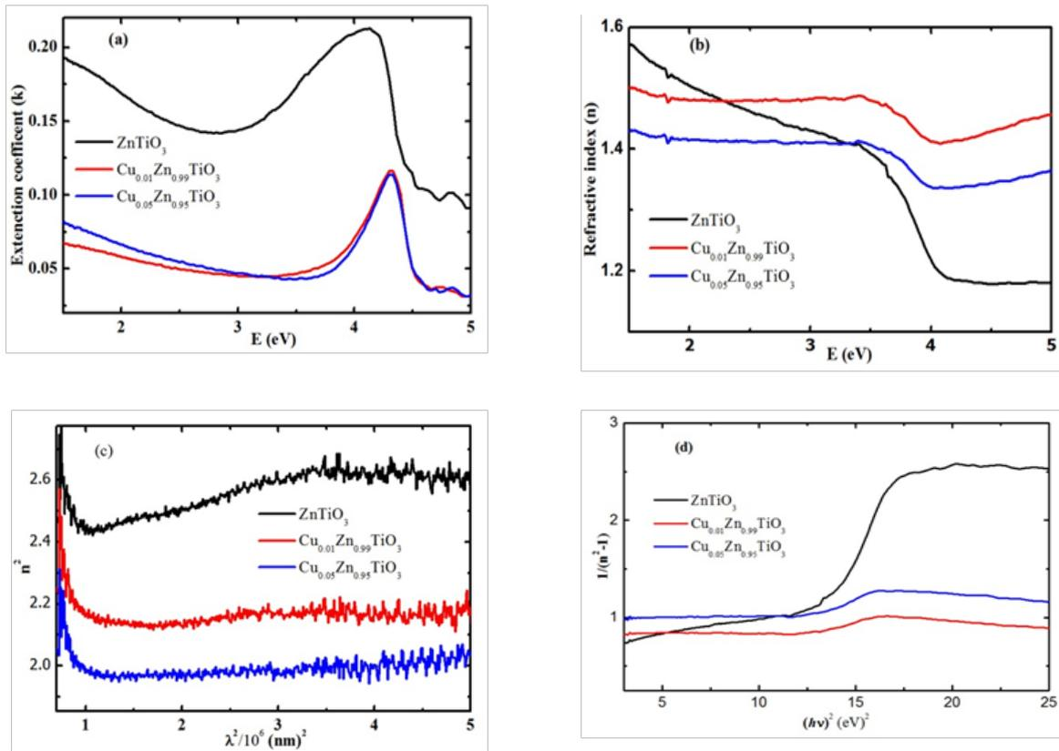
Fig. 5. (a) Extinction coefficient and (b) Refractive index as functions of wavelength. (c)  $n^2$  as a function of square wavelength. (d)  $1/(n-1)^2$  as a function of square photon energy for ZnTiO<sub>3</sub>, Cu<sub>0.01</sub>Zn<sub>0.99</sub>TiO<sub>3</sub> and Cu<sub>0.05</sub>Zn<sub>0.95</sub>TiO<sub>3</sub> thin films with thickness 250, 276, and 300 nm, respectively, deposited on glass substrates and annealed at 400 °C for 1 h.
