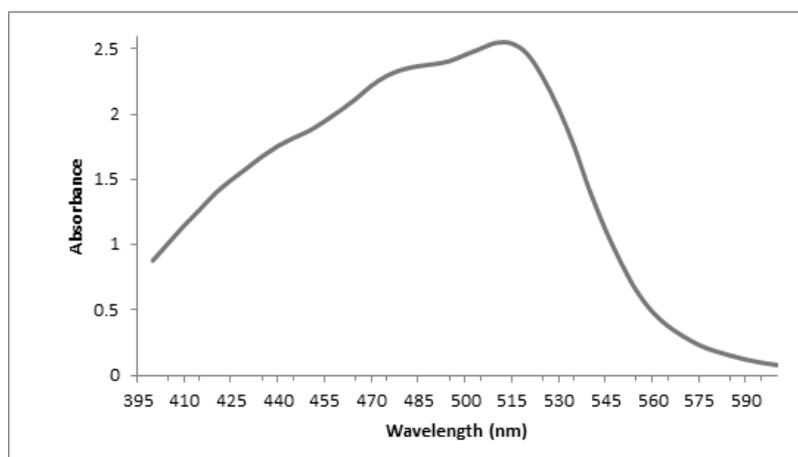
**Fig. 1. Absorption spectrum of ferriin indicator solution.**
