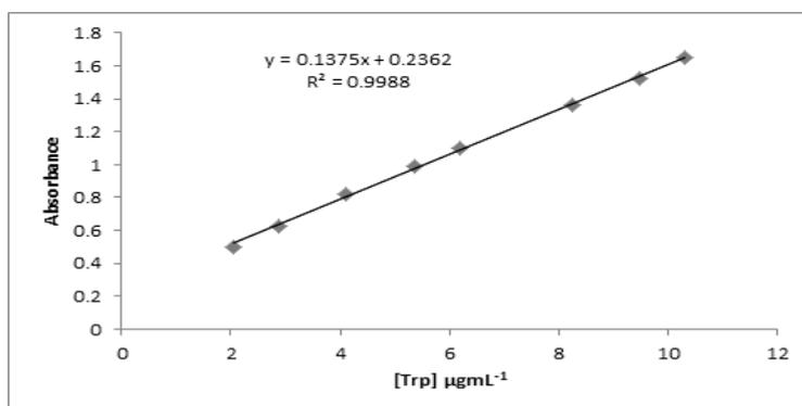
Fig.14. Calibration graph of the reaction between Trp in its oxidized form and Ferriin (II) at  $\lambda_{\max} = 515 \text{ nm}$ .
