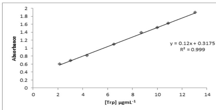
**Fig.16. Calibration graph of Trp in the synthetic mixture using [ferroin III] =  $2.0 \times 10^{-4}$  M at  $\lambda_{\text{max}} = 515$  nm.**
