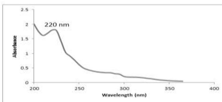
Fig. 12. Spectrum of  $1.004 \times 10^{-4}$  M Trp in  $0.3024$  N  $\text{H}_2\text{SO}_4$  medium.
