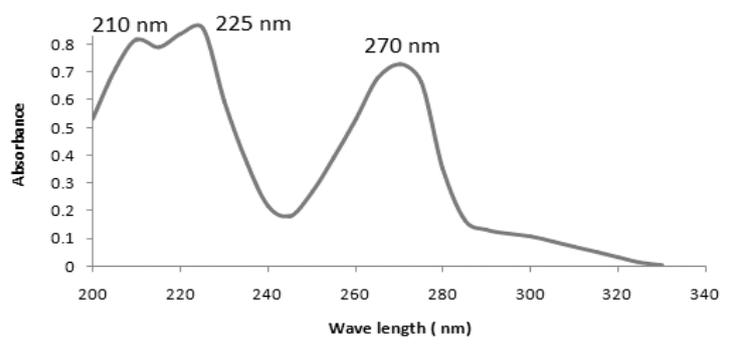
**Fig. 10.** The UV absorption spectrum of the ferrioxalate (II)-Trp oxidized form product ( $1 \times 10^{-5}$  M) at 135 min.
