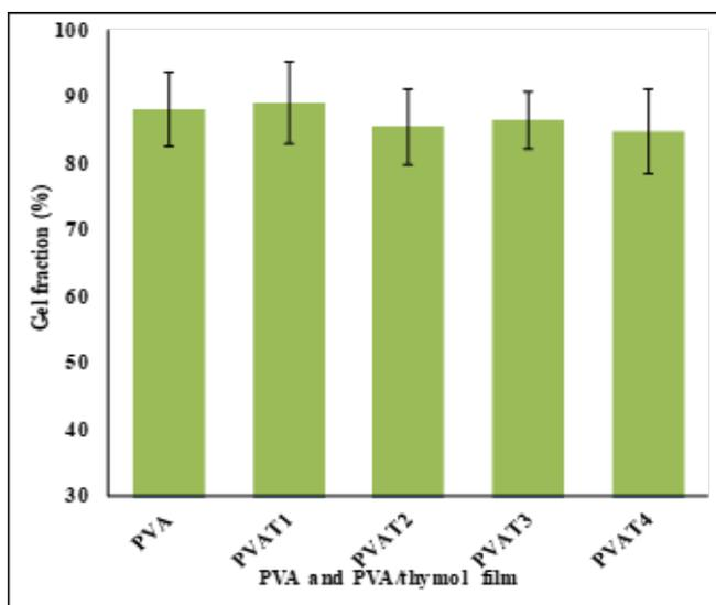
Fig. 6. Gel fraction of PVA, PVA/thymol film (PVA: PVA 8%; PVAT1:PVA 8% and thymol 0.125%; PVAT2:PVA 8% and thymol 0.25%; PVAT3:PVA 8% and thymol 0.5%; PVAT4:PVA 8% and thymol 1%)
