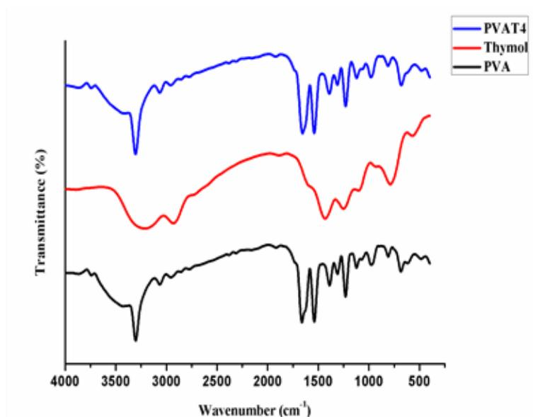
Fig. 1. FTIR spectra of PVA, PVA/thymol film and thymol (PVAT4: PVA 8% and thymol 1%).
