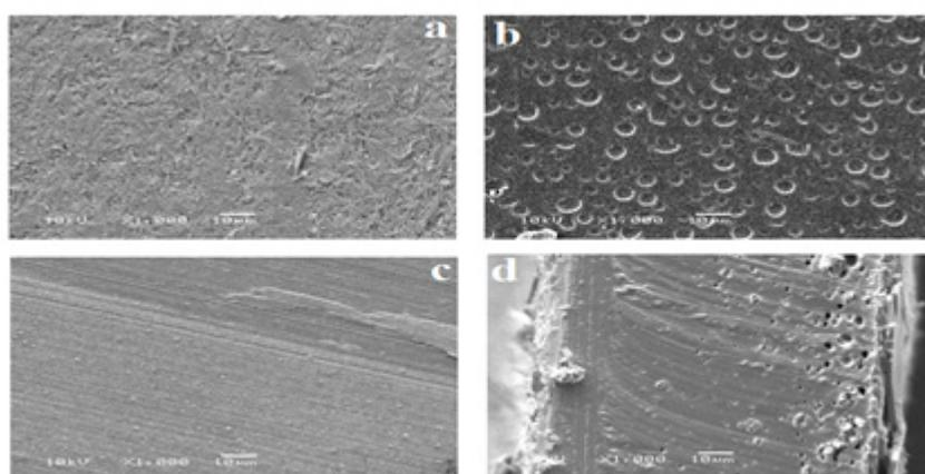
Fig.4. SEM micrograph of PVA, PVA/thymol film (PVAT4) (PVAT4: PVA 8% and thymol 1%).
