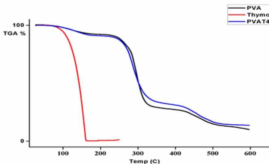
Fig. 3. TGA curve for of PVA, PVA/thymol film and thymol with heating
