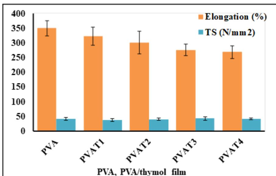
Fig. 5. Mechanical properties of of PVA, PVA/thymol film (PVA: PVA 8%; PVAT1:PVA 8% and thymol 0.125%; PVAT2:PVA 8% and thymol 0.25%; PVAT3:PVA 8% and thymol 0.5%; PVAT4:PVA 8% and thymol 1%)
