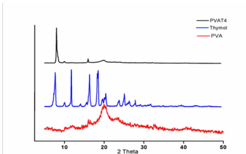
Fig. 2. X-ray diffraction (XRD) patterns of PVA, PVA/thymol film and thymol (PVAT4: PVA 8% and thymol 1%).
