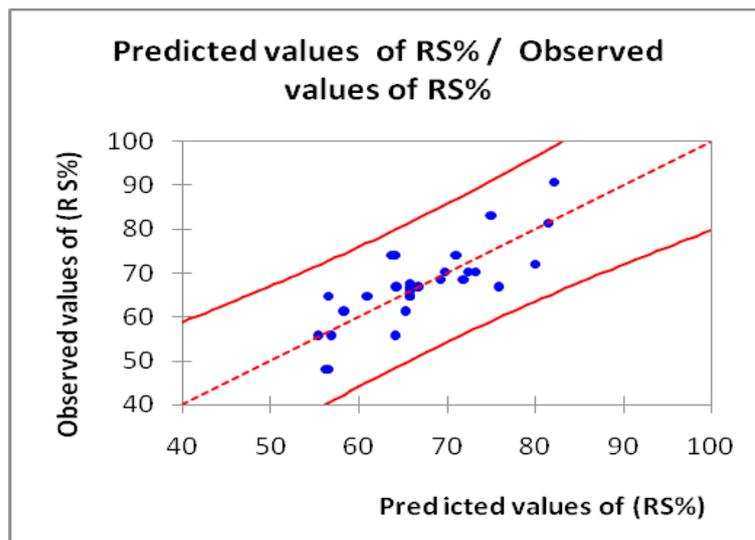
Fig. 7. Correlation between the observed and predicted values for RS (%) determined by the first-order polynomial equation.
