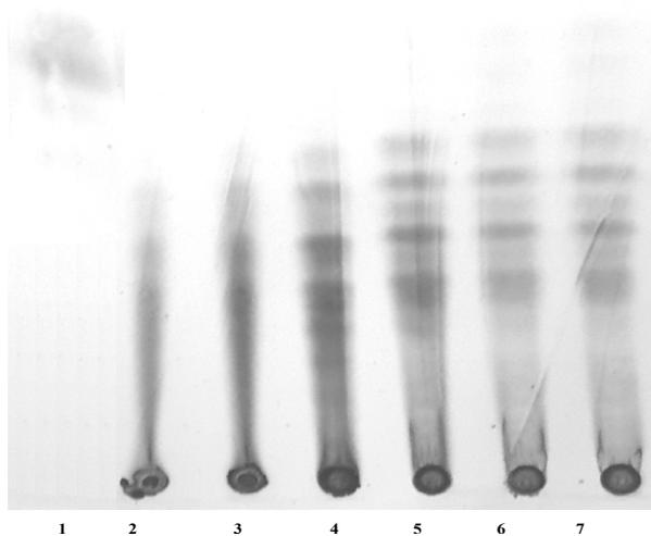
**Fig. 5.** TLC plate of chitooligosaccharides produced by the hydrolysis of soluble chitosan by chitosanase. Lan 1: glucosamine. Lan 2-9: represent the hydrolysis products different E/S ratio 0.0125, 0.025, 0.05, 0.1, 0.15 and 0.2 respectively.
