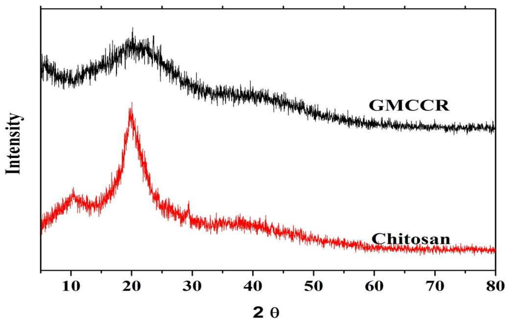
Fig. 3. The XRD spectrum of chitosan and GMCCR resin
