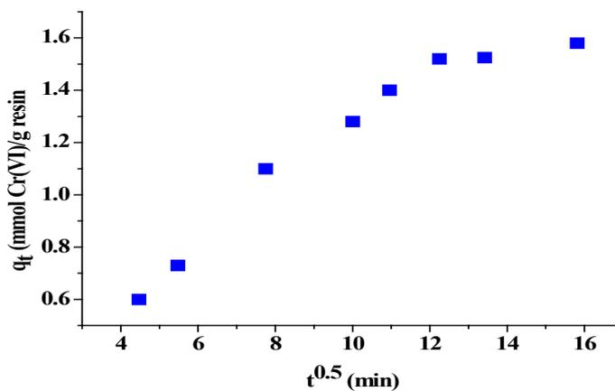
Fig. 10. The intraparticle diffusion kinetic model of the uptake of Cr(VI) by (GMCCR)
