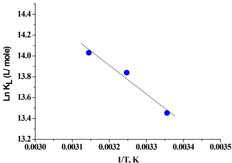
Fig. 7. Van't Hoff plots for adsorption of Cr (VI) on Chitosan-Glycine resin.
