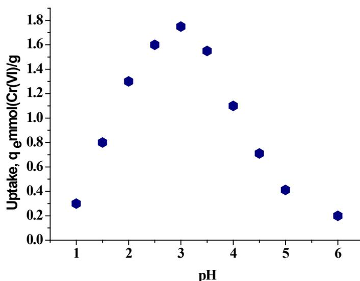
**Fig. 4.** Effect of pH on the uptake of Cr (VI) by Chitosan-Glycine resin at initial concentration of  $5 \times 10^{-3} \text{ M}$  for; contact time 150 min at temperature 25°C.
