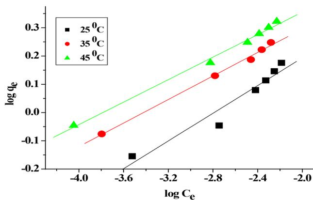
Fig. 6. Freundlich isotherms for the adsorption of Cr (VI) on (GMCCR) at different temperatures; pH 3; contact time 150 min.
