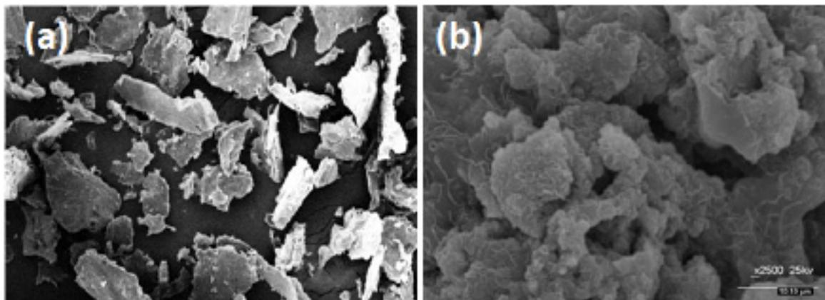
Fig. 2. SEM micrographs of a) chitosan and b) GMCCR resin (the surface morphology)
