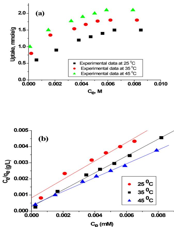
Fig. 5.a) Uptake Cr (VI) on (GMCCR) at different temperatures; pH 3; contact time 150 min, b) Langmuir isotherm.isotherm.
