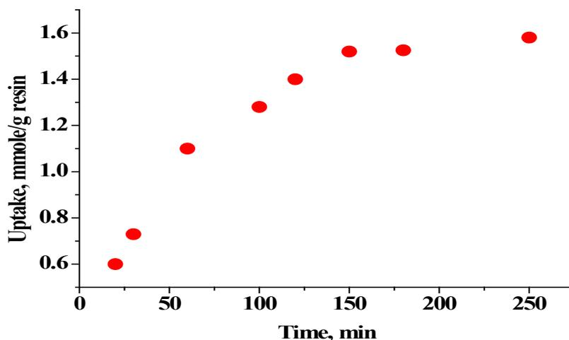
Fig. 8. Uptake of Cr (VI) by Chitosan-Glycine resin as a function of time at 25°C; pH 3; initial concentration of  $5 \times 10^{-3}$  M.
