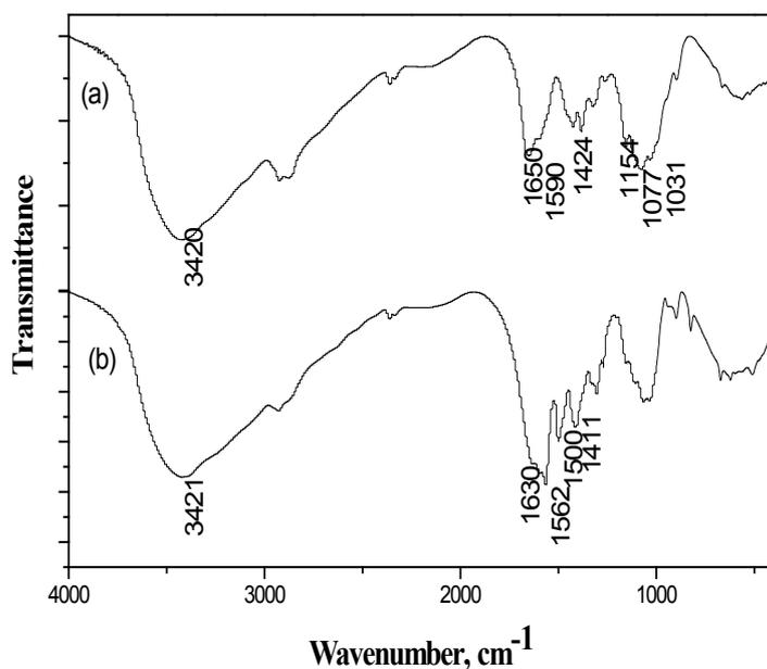
Fig. 1. FTIR of a) chitosan and b) glycine modified chosen resin(GMCCR).
