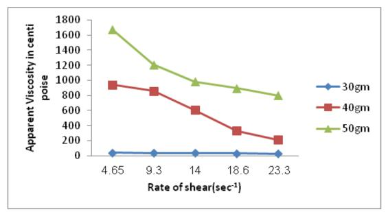
Fig.1. Dependance of the apparent viscosity on the rate of shear .
