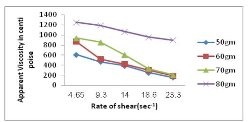
Fig. 2 . Dependance of the apparent viscosity on the concentration of urea and rate of shear. Egypt. J. Chem. 63, No. 9 (2020)
