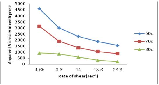
Fig.5. Dependance of the apparent viscosity on temperature and rate of shear.
