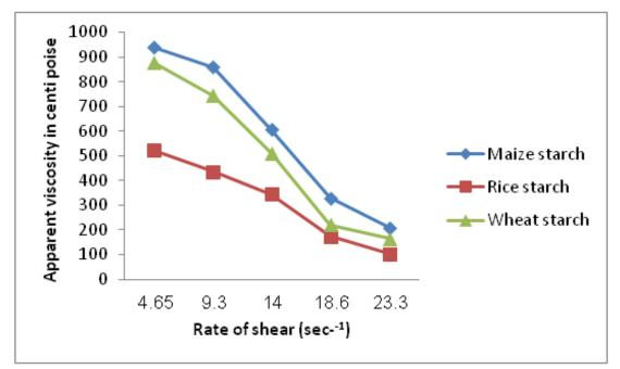
Fig.7. Dependence of the apparent viscosity on Type of starch and rate of shear.
