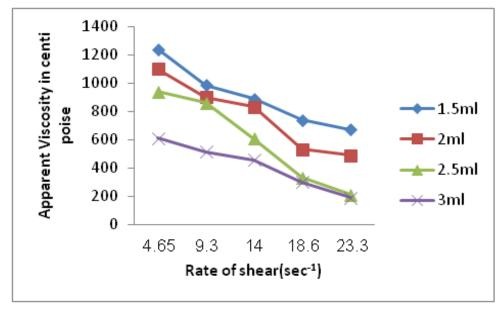
Fig.3 Dependance of the apparent viscosity on the concentration of enzyme and rate of shear.
