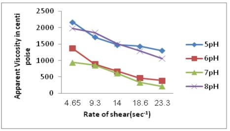
Fig.4. Dependance of the apparent viscosity on pH and rate of shear.
