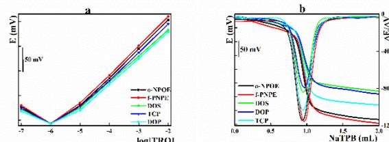
**Fig. 3.** Effect of the membrane plasticizer on: a) TR sensor performance; b) potentiometric titration of 1 ml of 10<sup>-2</sup> mol L<sup>-1</sup> TR with 10<sup>-2</sup> mol L<sup>-1</sup> NaTPB solution.
