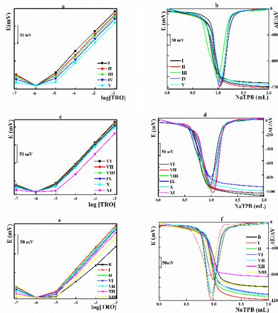
**Fig. 1:** a, c, e ) Effect of the ionophores on TRO sensor performance, b, d, f ) potentiometric titration of 1 ml of  $10^{-2}$  mol L<sup>-1</sup> TRO with  $10^{-2}$  mol L<sup>-1</sup> NaTPB solution.
