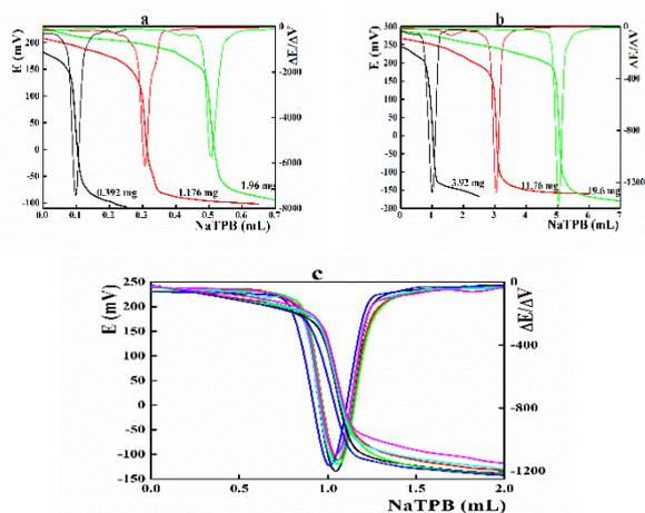
Fig. 6 : a, b) Potentiometric titration of different TRO concentrations against  $10^{-2}$  mol L<sup>-1</sup> NaTPB, c) reproducibility of titration for 1 ml of  $10^{-2}$  mol L<sup>-1</sup> TRO solution with  $10^{-2}$  mol L<sup>-1</sup> NaTPB solution.
