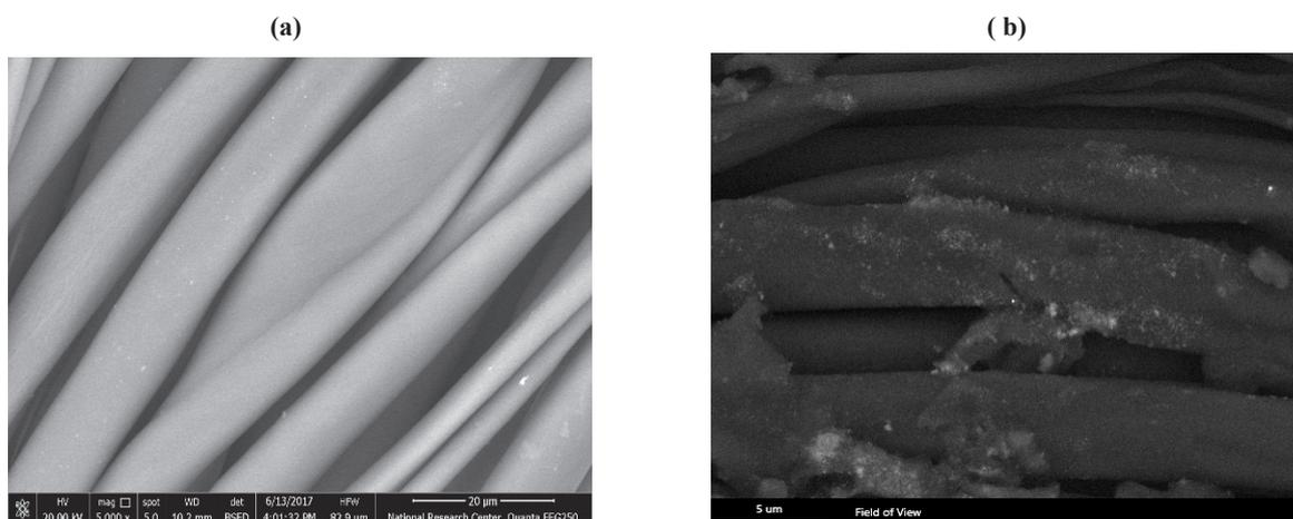
Fig. 1. SEM images of the untreated(a) and treated(b) polyester with caustic soda. [Conc. = 60 g/dm<sup>3</sup>, 100 °C, 65min].
