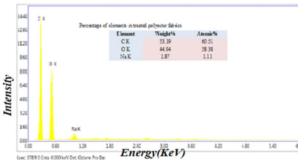
Fig. 3. EDX analysis of treated polyester fabric with caustic soda [C =  $60\text{ g/dm}^3$ ,  $100^\circ\text{C}$ , 65min].
