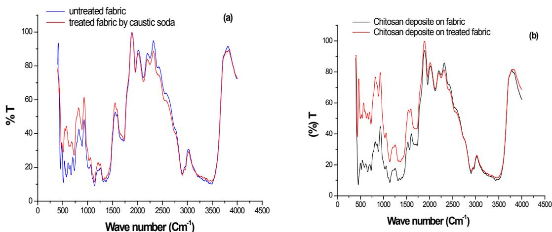
Fig. 4. FT-IR spectrum for untreated and treated polyester/ cotton blend fabric with (a) caustic soda [C =  $60\text{ g/dm}^3$ ,  $100^\circ\text{C}$ , 60 min] (b) chitosan [  $7\text{ g/dm}^3$ ,  $25^\circ\text{C}$ , 60 min].
