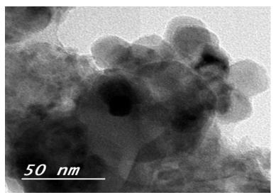
Fig. 3. EM analysis of Synthesized GO nanostructures
