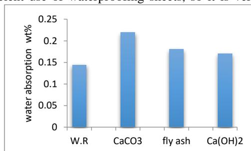
important to determine the water absorption percent after 24 h immersion as shown in Fig. (2) for the different filler samples and for the rubber with different Waste rubber concentrations (while no effect on water absorption coefficient when waste oil was used), according to ASTM (D570) [10]:
