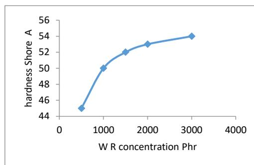
Fig (4) Hardness for different filler types and for WR filler.
