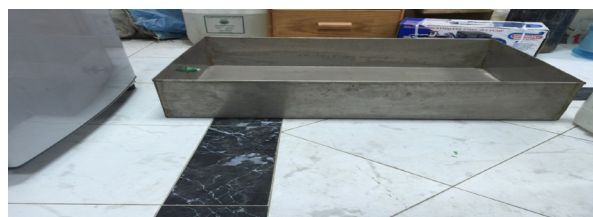
Fig. 2. 50 litres exposed stainlesssteel 316 solar pond.
