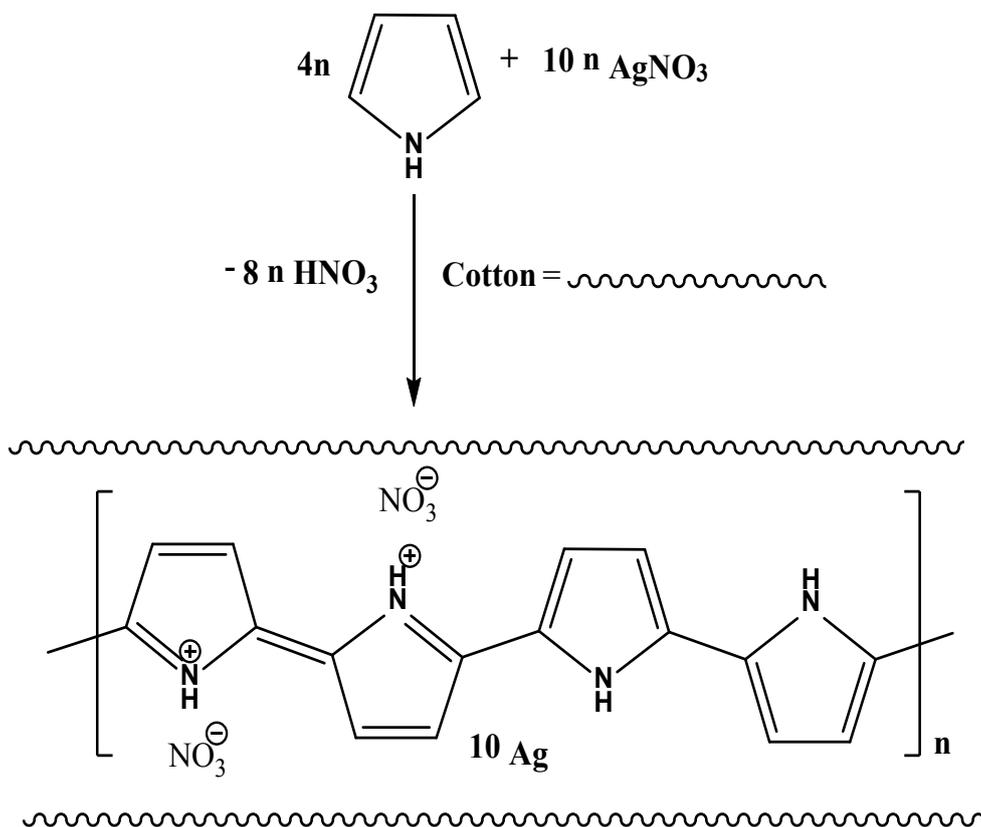
**Fig 1.** In situ coating of cotton fabric with Ag/PPy nanocomposite.
