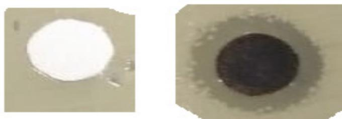
**Fig. 5. A representative antibacterial image of the inhibition zone for Ag/PPy-nanocoated cotton fabric (right) compared with the uncoated one (left). The inhibition zone due to anti *Escherichia coli*.**
