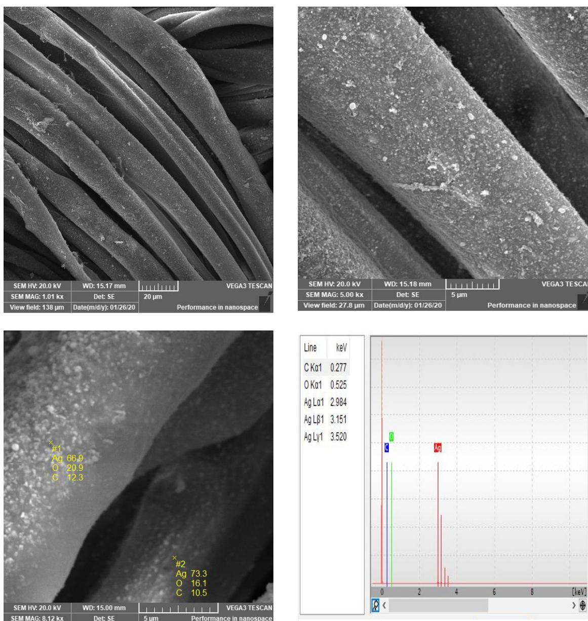
Fig. 3. SEM images of Ag/PPy-nanocoated cotton fabrics with different magnifications. The images below from left to right show the EDX analysis at two different points and the spectrum at any point.
