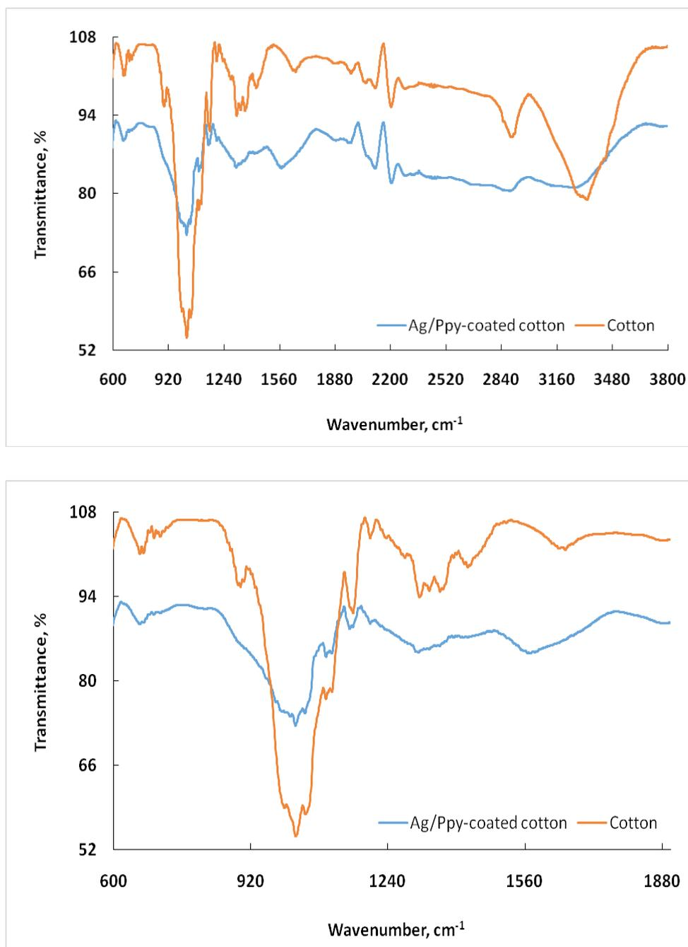
Fig. 2. ATR-FTIR spectra of Ag/PPy-nanocoated cotton and cotton fabrics. The upper figure is full scale and the lower one is an expanded region.
