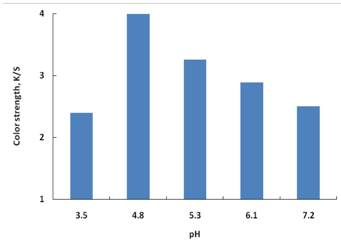
Fig. 4. Effect of the print paste pH on the color strength the printed fabric.
