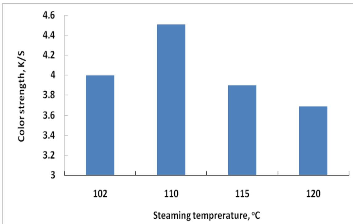
Fig. 6. Effect of steaming temperature on the color strength the printed fabric.
