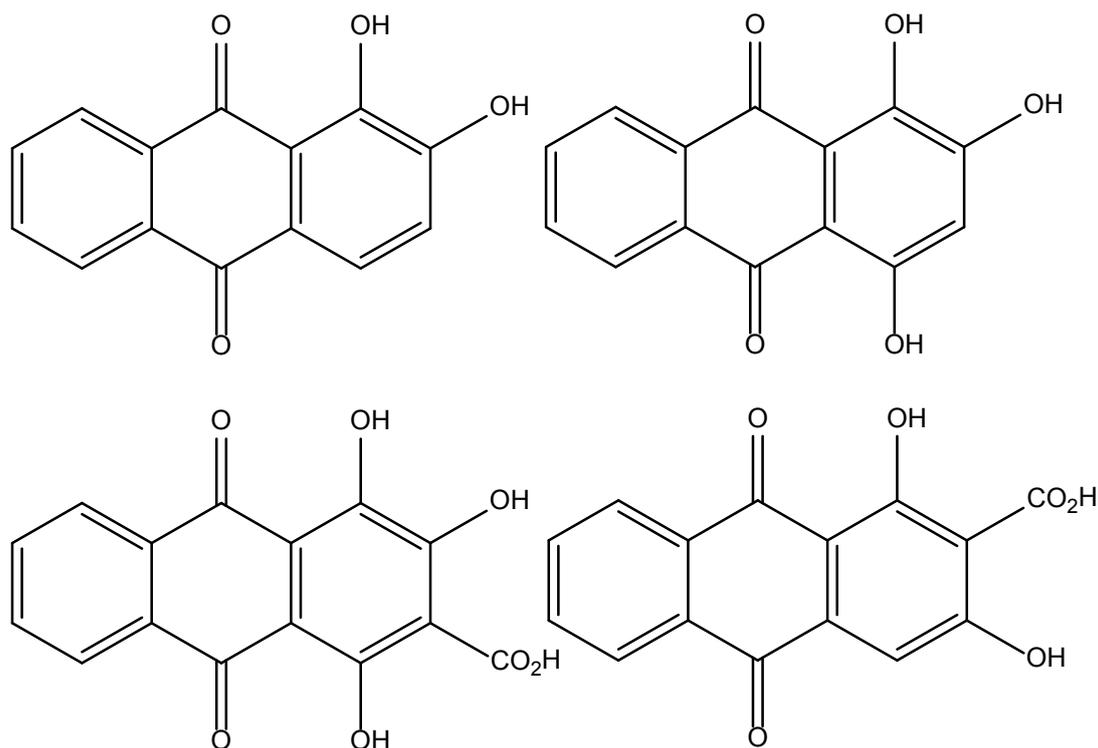
Fig. 1. Main coloring components of madder natural dye,
