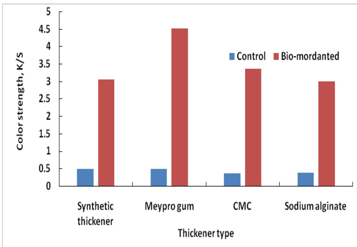
Fig. 7. Effect of thickener type on the color strength of the printed fabric.
