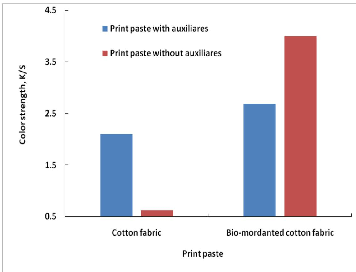
Fig. 3. Effect of the print paste formulation on the color strength the printed fabric.
