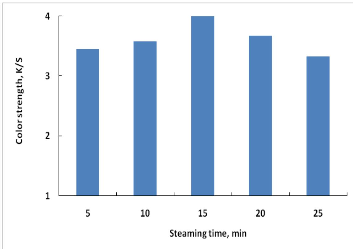
Fig. 5. Effect of steaming time on the color strength the printed fabric.
