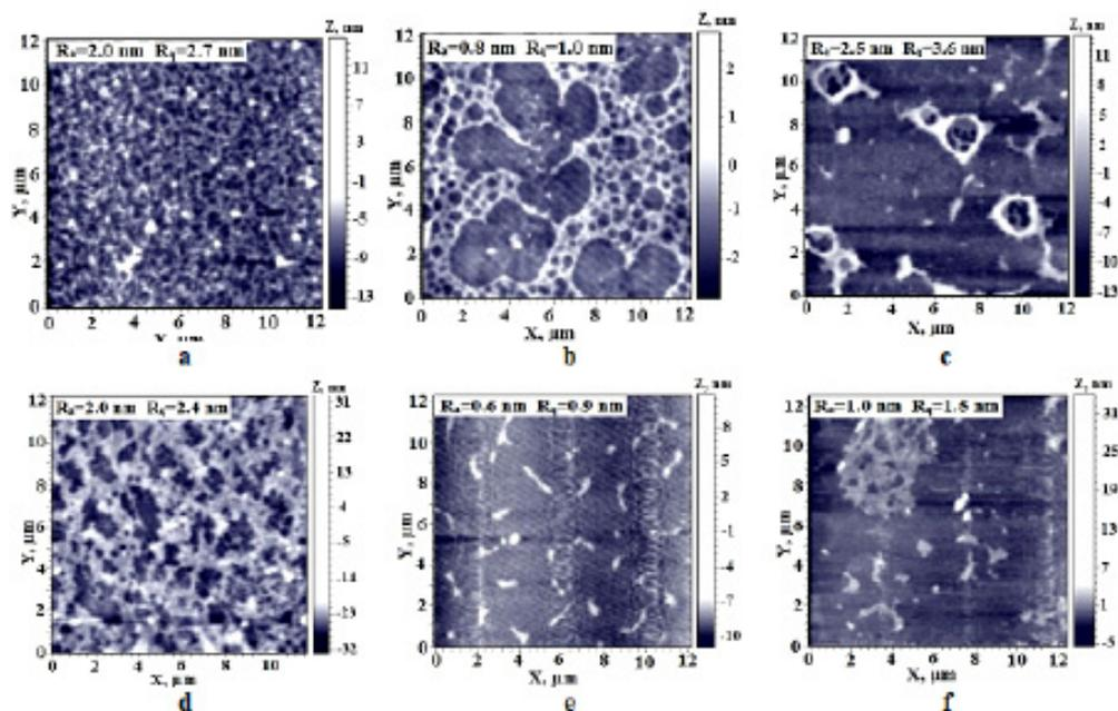
**Figure 7.** AFM height images of the surface of a double emulsion thin film 5-FU-PCL/PVA containing 1% by weight of a 5-FU preparation cast on mica; ratio of PCL: PVA: a- (1: 0.5), b-(2:0.5), c-(3:0.5), d- (1:1), e- (2:1), f- (3:1).
