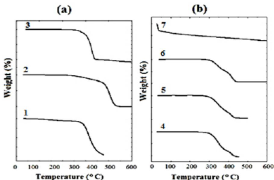
**Figure 5.** TGA thermograms of (a): 5-FU (3), PCL (2), PVA (1) and (b):5-FU-PCNs formulations F3:0.5 (4), F3:1 (5), F3:3 (6) and F2:1 (7), respectively.
