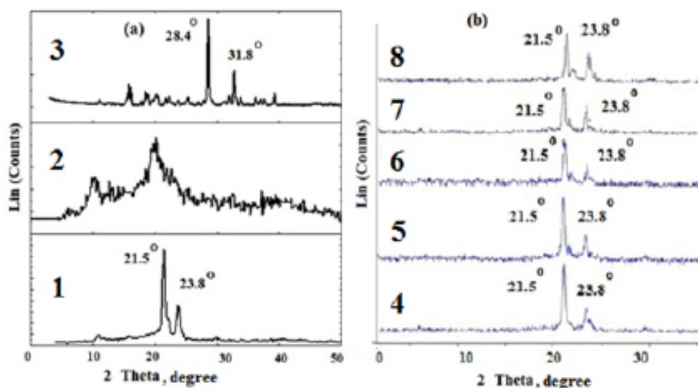
**Figure 2.** XRD patterns of (a) pure PCL (1), PVA (2), 5-FU (3), and (b) 5-FU-PCNs formulations F2:0.5 (4), F3:0.5 (5), F1:1 (6), F2:1 (7) & F3:1 (8), respectively.
