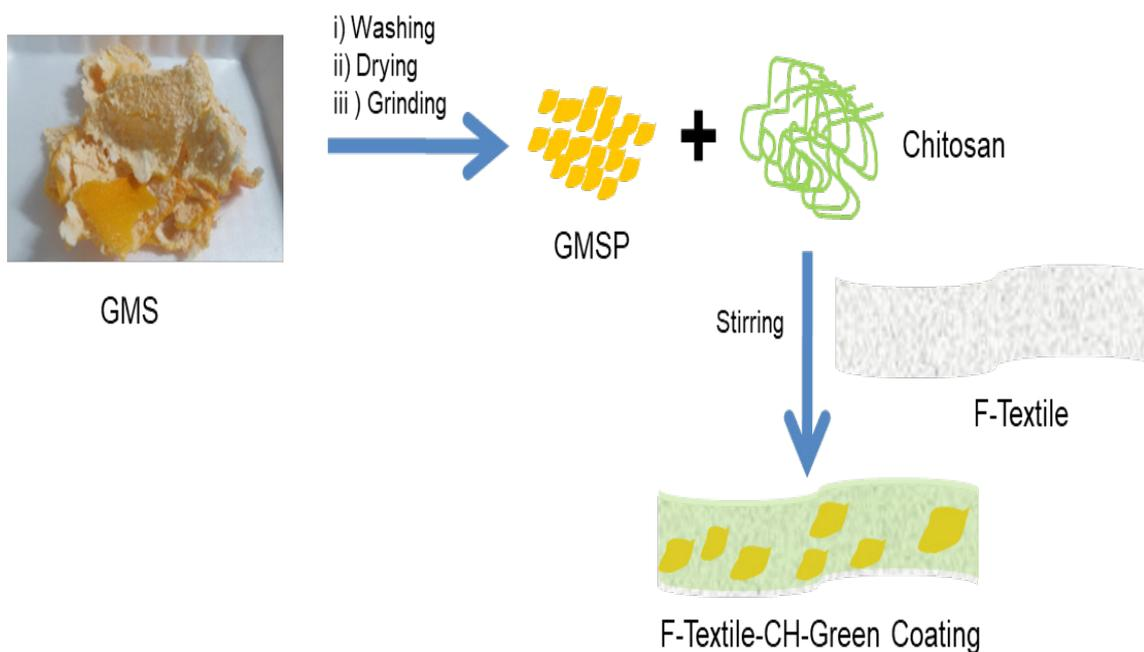
Fig. 1. Schematic diagram representing the synthesis of green mandarin peel powder based textile coating.
