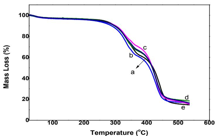
Fig. 3. TGA graphs blank furniture textile fabrics (a) F-CH-GMPP 20 (b), F-CH-GMPP 30(c), F-CH-GMPP 50 (d) and F-CH-GMPP 70(e).
