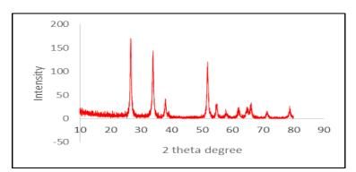
Fig. 4c. XRD patterns of SnO<sub>2</sub> NPs.
