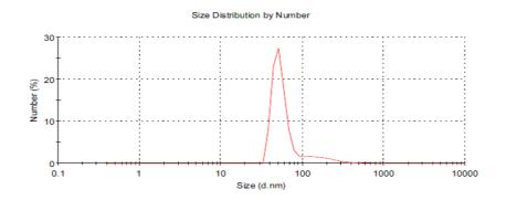
Fig. 5b. Particle size distribution of SnO<sub>2</sub>NPs.
