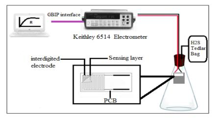
Fig. 2. The experimental setup for gas monitoring with Interdigited electrode design.
