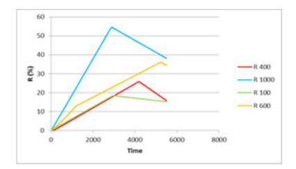
Fig. 9. The dynamic sensing response of  $Ppy/SnO_2$  sensor towards different concentrations of  $H_2S$  gas with time.
