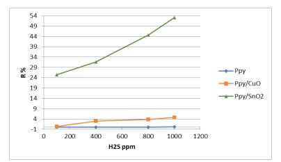
Fig. 8. The sensing response of Ppy, Ppy/CuO and Ppy/SnO<sub>2</sub> sensor towards different concentrations of H<sub>2</sub>S gas.
