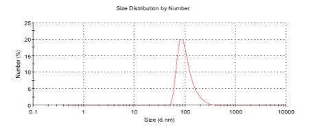
Fig. 5a. Particle size distribution of CuO NPs.
