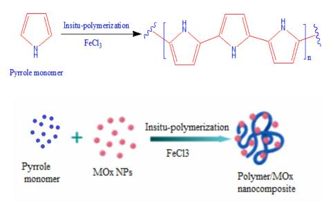
Fig. 1. Scheme of polymerization reaction.
