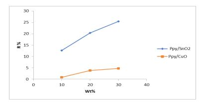
Fig. 7. The 100 ppm H<sub>2</sub>S gas response of different doping ratios of NPs to Polypyrrole.
