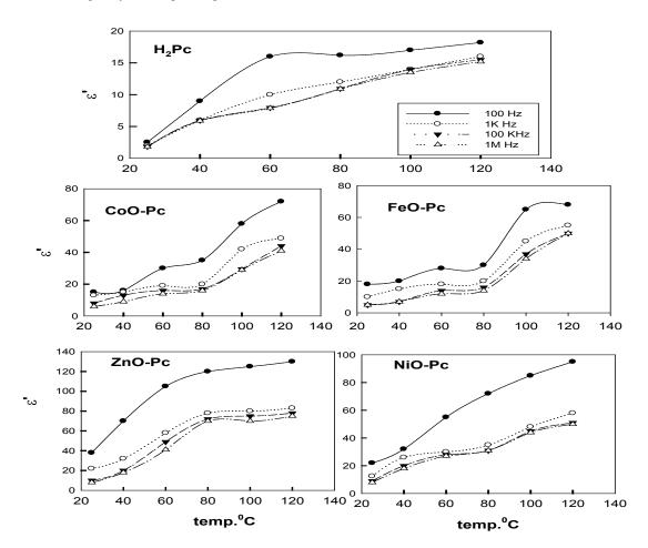
Fig.5.Variation of dielectric constant ɛ' with temperature at different frequencies for H2Pc and different MO-Pc.
