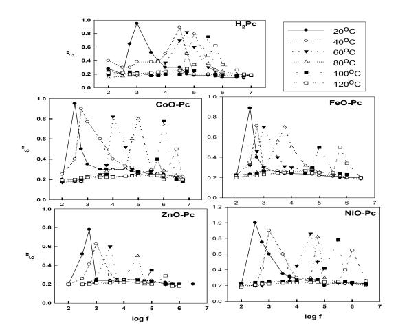
Fig.7. Variation of dielectric loss ɛ'' with frequency at different temperature for H2Pc and MO-Pc.
