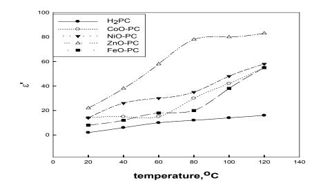
Fig.6.Variation of dielectric constant with temperature at 1000Hz for H2Pc and MO-Pc.
