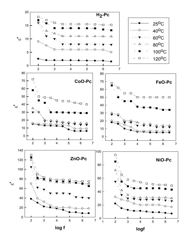
Fig.4. Variation of dielectric constant  $\epsilon'$  with frequency at different temperatures for H2Pc and MO-Pc.
