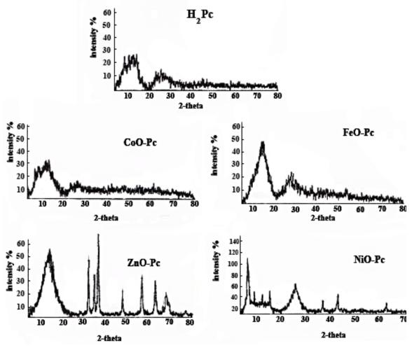
Fig. 3. XRD spectra of H2Pc and MO-Pc composites.
