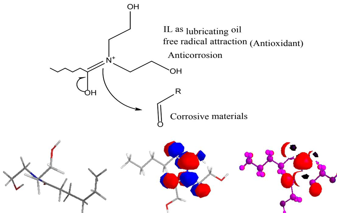
**Fig. 7. outline the electronic distribution of the amide-enaminol isomers that responsible for scavenging the free radical and corrosive materials**
