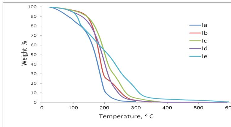
Fig. 8. Thermal gravimetric analysis for the prepared ILs (Ia-Ie).
