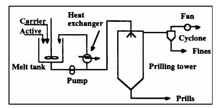
Fig. 23. Spray chilling (Prilling) [53].
