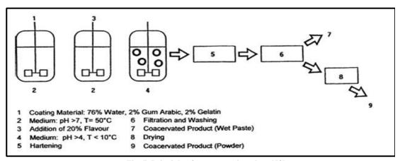
Fig. 7. Principle of a coacervation plant [58].
