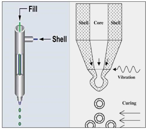
Fig. 27. The Co-extrusion process [81].
