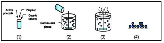
Fig. 9. Basic steps of microencapsulation by solvent evaporation [60].
