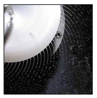
Fig. 28. Encapsulation by spinning disc [12,25].
