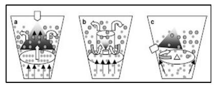
Fig. 21. Styles of a fluid-bed coating (a) Top spray, (b) bottom spray, (c) tangential spray [34].
