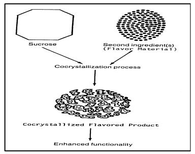
Fig. 29. Flow diagram of encapsulation cocrystallization process [83].
