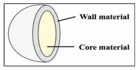
Fig. 1. Schematic presentation of the capsule structure [8].
