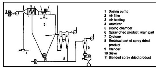
Fig. 13. Principle of a spray drying plant [58].
