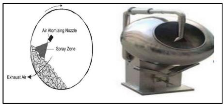
Fig. 25. Representation of a typical pan coating [34].
