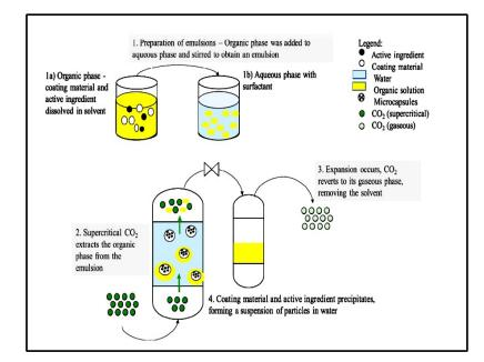
Fig. 11. Schematic representation of supercritical fluid extraction of emulsions (SFEE) [61].
