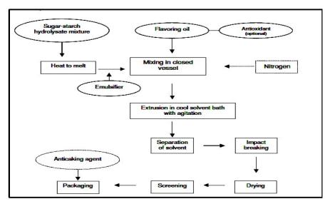
Fig. 26. Flow diagram of encapsulation of food flavors by extrusion [32].
