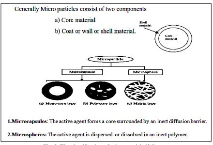
Fig. 2. The classification of microparticle [34]
