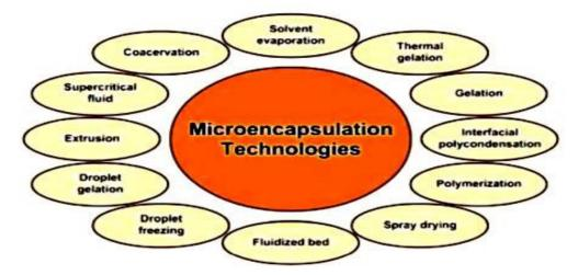
Fig. 6. Microencapsulation techniques [34].
