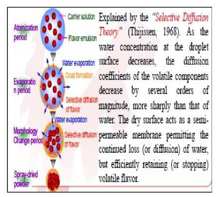
Fig. 18. Flavor retaining mechanism [10].
