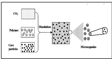
Fig. 10. Encapsulation by supercritical solutions rapid expansion [34].
