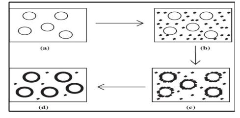
Fig. 8. Coacervation process; (a) Core material dispersion in solution of shell polymer; (b) Separation of coacervate from solution, (c) Coating of core material by micro droplets of coacervate; (d) Coalescence of coacervate to form continuous shell around core particles [34].
