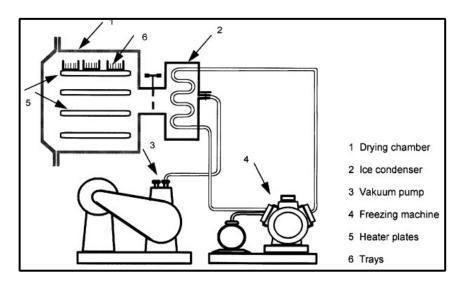
Fig. 24. Freeze-drying [75].
