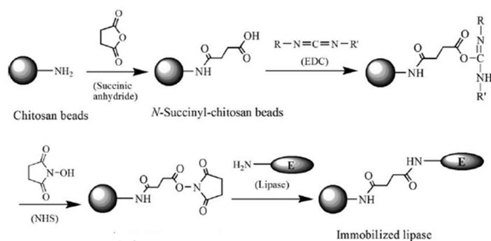
Figure 2: EDC-NHS activation of N-succinyl-CS beads [65].
