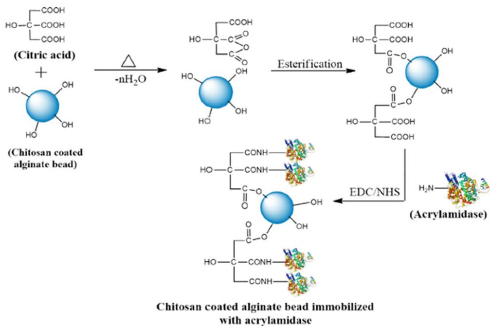
Figure 6: EDC-NHS activation of citric cross-linked CS encrusted Alg beads [12].
