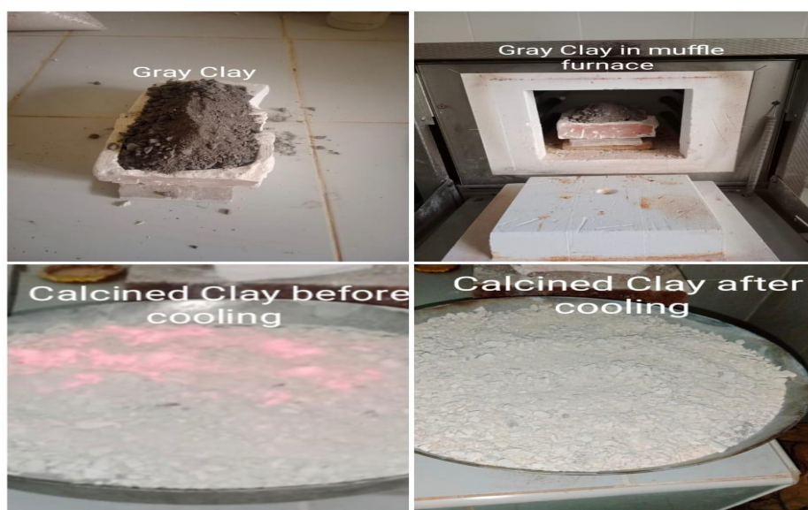
Figure 1: Calcination processes of gray clay.
