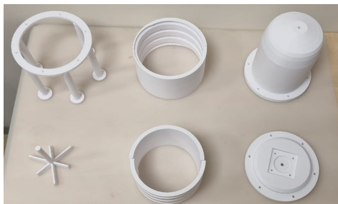
Figure 5 - AM-based reactor components (main body with heat exchanger and mixer)
