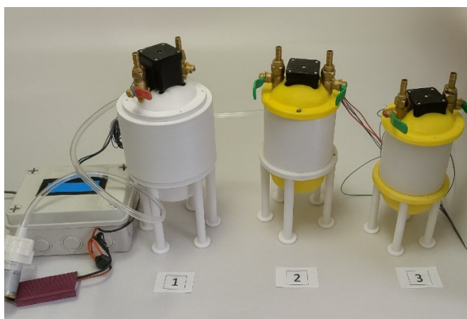
Figure 6 - Additively manufactured continuous-flow reactor system for biphenyl synthesis
