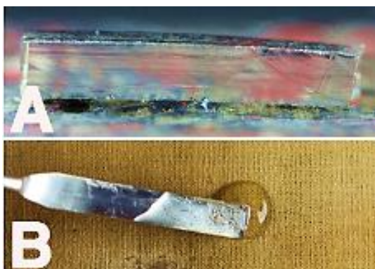
Fig 4. Gels used in cleaning: (A) a rigid gel (gellan gum); (B) a soft gel (Klucel™) [82].
