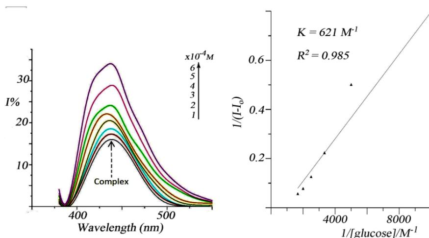
Fig. 5 Fluorescence spectra of the complex  $[\text{NdL}^4(\text{NO}_3)_2(\text{H}_2\text{O})_3] \cdot 4\text{H}_2\text{O}$  ( $10^{-4}$  M) in presence of increasing amounts of glucose ( $1 \times 10^{-4}$  M– $7 \times 10^{-4}$  M) using phosphate buffer (pH 7.4).
