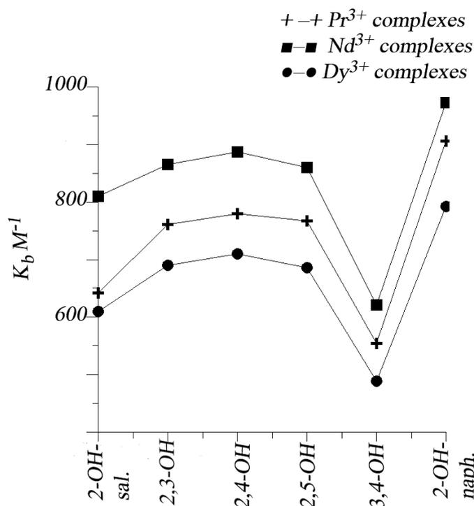
Fig. 6(b). Effect of OH position in the MF Schiff-bases of the  $K_b$  values of the  $\text{Pr}^{3+}$ ,  $\text{Nd}^{3+}$  and  $\text{Dy}^{3+}$  complexes from emission spectroscopy.
