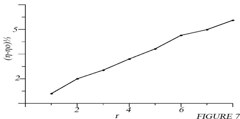
Fig. 7. Effect of increasing amounts of glucose ( $1 \times 10^{-4} \text{M}$ – $8 \times 10^{-4} \text{M}$ ) on the viscosity of the  $[\text{NdL}^1(\text{NO}_3)_2(\text{H}_2\text{O})_3] \cdot 2\text{H}_2\text{O}$  complex ( $10^{-4} \text{M}$ ) in phosphate buffer ( $\text{pH}=7.4$ ).
