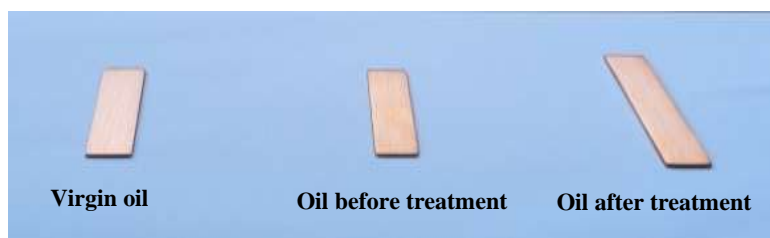
Fig. 14. Copper Strips with different oils (virgin oil, oil before and after treatment).
