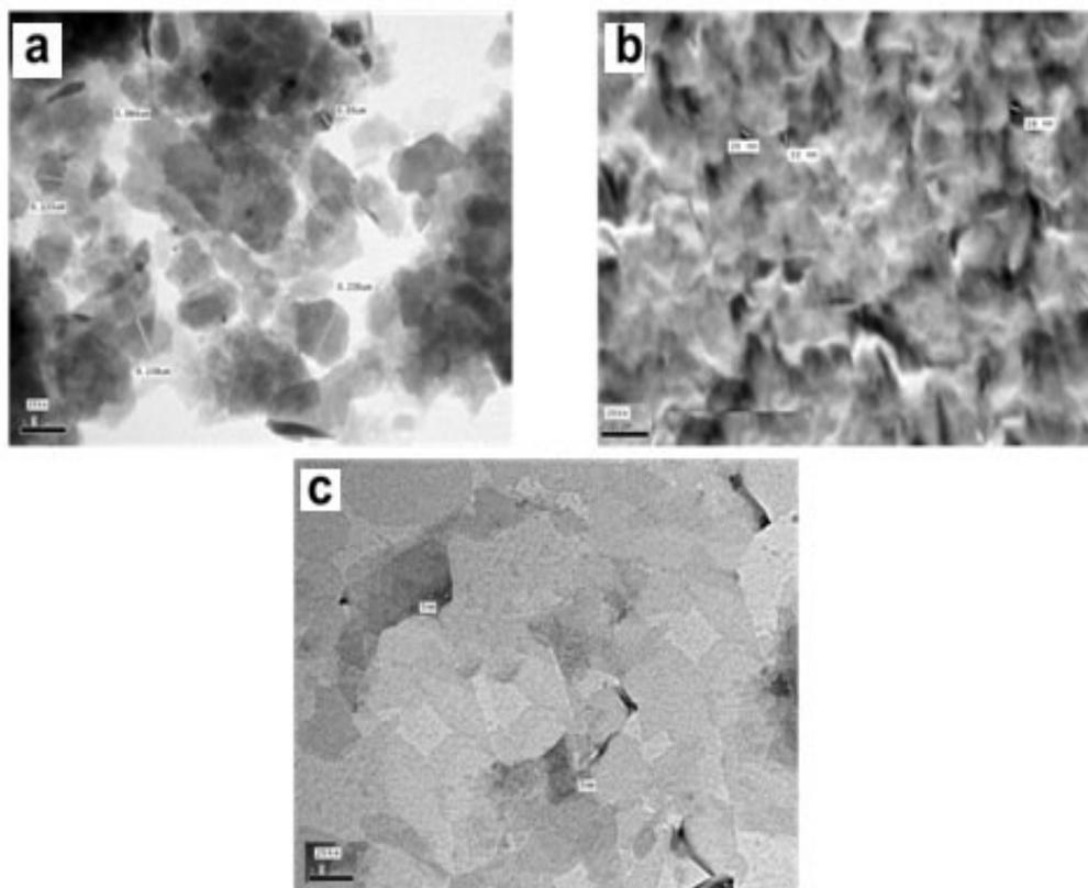
**Fig. 3. TEM micrographs of: (a) unmodified bentonite (SB), (b) pretreated bentonite (PSB) with distilled water and (c) modified bentonite (MSB) with non-ionic surfactant (Tween-80)**
