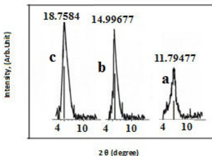
**Fig. 2. (a) XRD patterns unmodified bentonite (SB), (b) pretreated bentonite (PSB) with distilled water and (c) modified bentonite (MSB) with non-ionic surfactant (Tween-80)**
