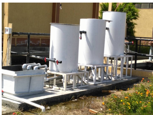
Fig. 3. The constructed pilot plant for the recycling of the sand filter “backwashing” water.
