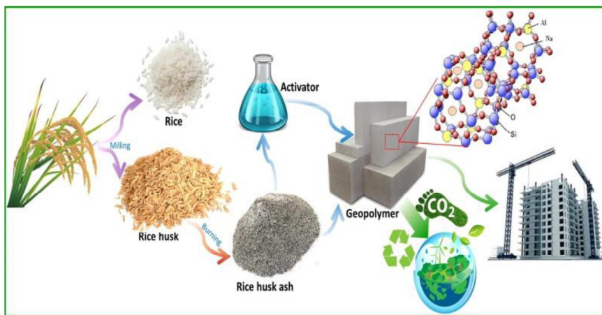
Figure 6: Rice husk ash–geopolymer construction [100].
