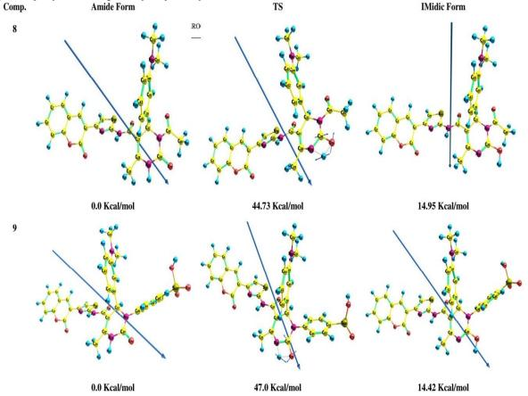
Figure 7. The optimized geometry, numbering system, vector of dipole moment, relative energy with respect to Amide form of the newly synthesized Coumarin compounds (8 and 9) with TS imaginary normal mode localized H34-N29-C30-O39 using B3LYP/6-311++g(d,p) level of calculation.
