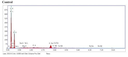
Fig. 2. Energy dispersive X-ray analysis (EDXA) of C1, C2, C3 and Control.
