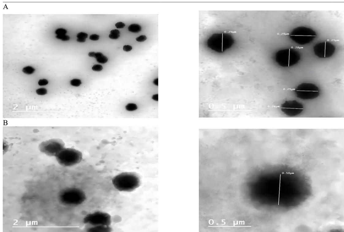
**Figure 2: TEM images of blank ethosomes (A) and insulin loaded ethosomes (B) Encapsulation Efficiency**
