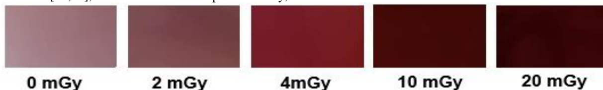
Figure 2. The color change in PVA/HX films after direct exposition to various \gamma -ray doses.
