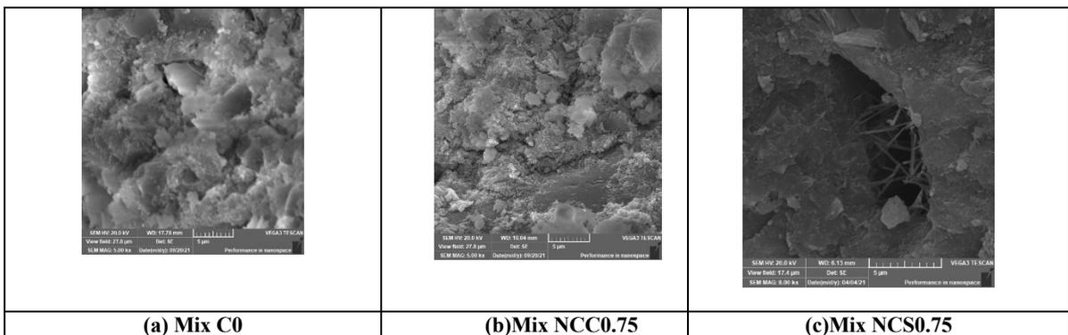
Fig. 6: SEM at 28 days for mixes (a) C0, (b) NCC0.75, (c) NCS0.75
