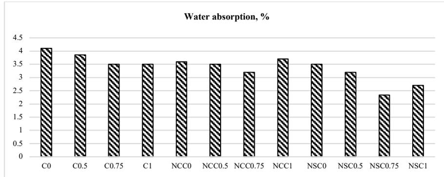
Fig. 5: Absorption Test for all mixes at 28 days
