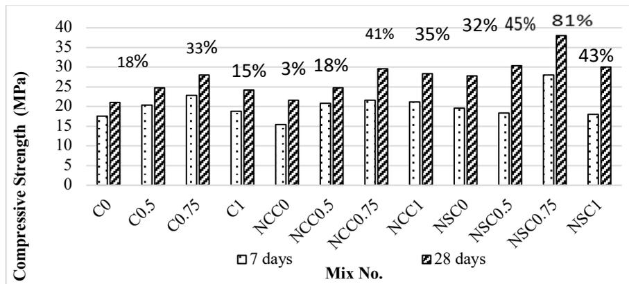
Fig. 1: Compressive Strength Results
