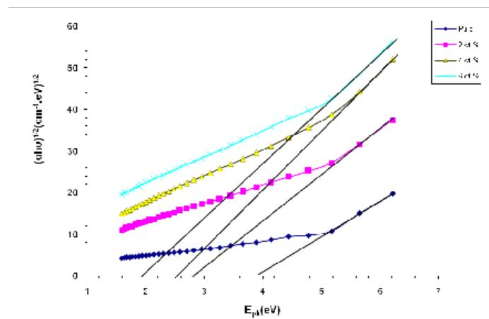
**Fig. 3.** Energies gaps for allowed indirect transition of PVA/SiO<sub>2</sub> nanocompsites.
