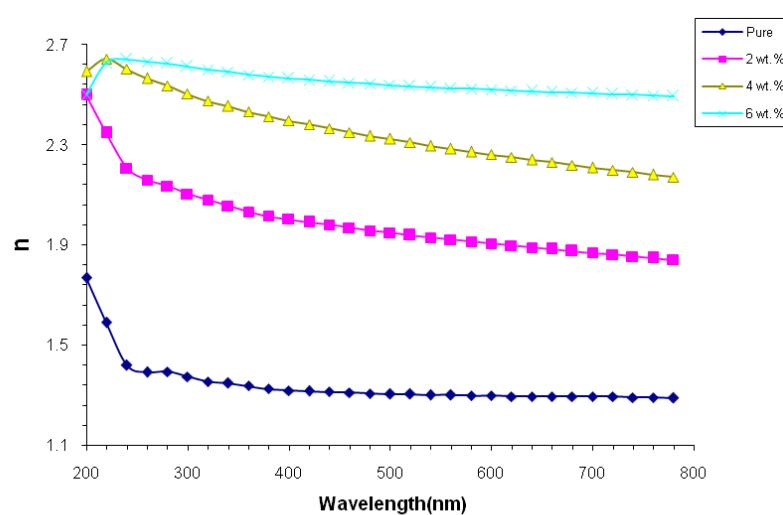
**Fig. 6. Variation of refractive index with photon wavelength for (PVA-SiO<sub>2</sub>) nanocomposites.**
