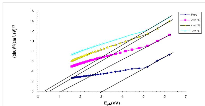
**Fig. 4.** Energies gaps for forbidden indirect transition of PVA/SiO<sub>2</sub> nanocompsites.
