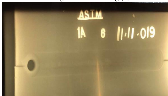
Fig. (3) Shows radiographic films for the dissimilar joint between Monel 400 and AISI1020 Carbon Steel using friction stir welding
