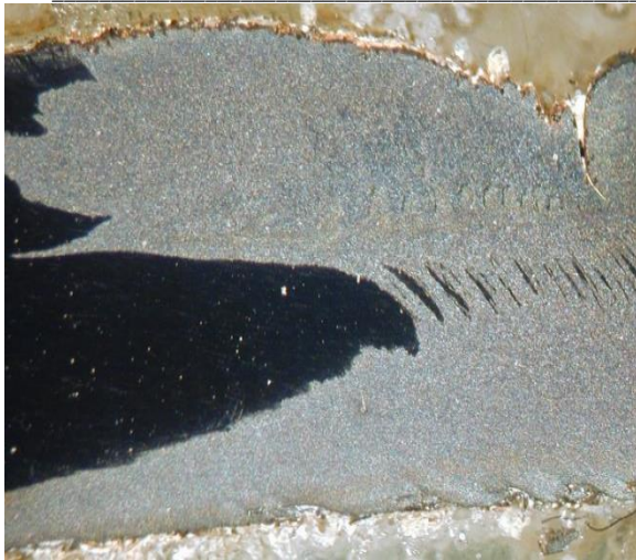
Fig. (5) FSW joining zones of Monel 400 with AISI 1020 Carbon Steel.
