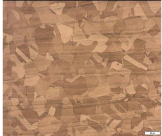
Fig.2 Microstructure of Monel400
