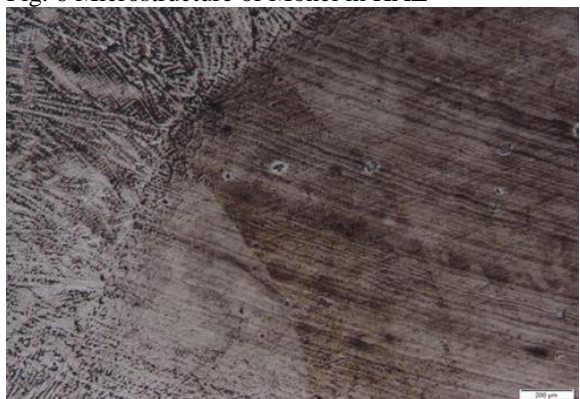
Fig. 7 Microstructure of Carbon steel in HAZ
