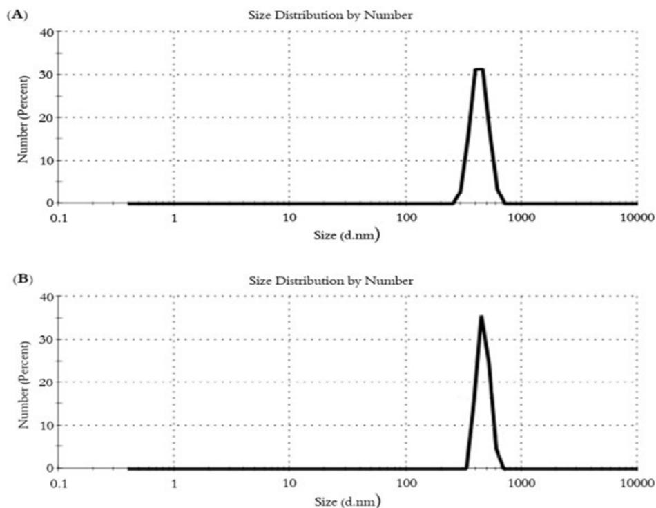
**Figure 3:** Nano-formulations particle size (A) ZnO with a size of  $433.2 \pm 19.46$  nm; (B) ZnO + *Citrus cinensis* nanoparticle formulation with a size of  $458.4 \pm 21.23$  nm.
