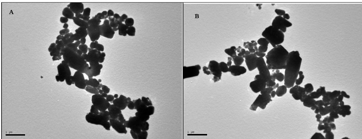
**Figure 5:** Transmission electron micrograph (TEM) of ZnO NPs (A) and ZnO with essential oil NPs (B).
