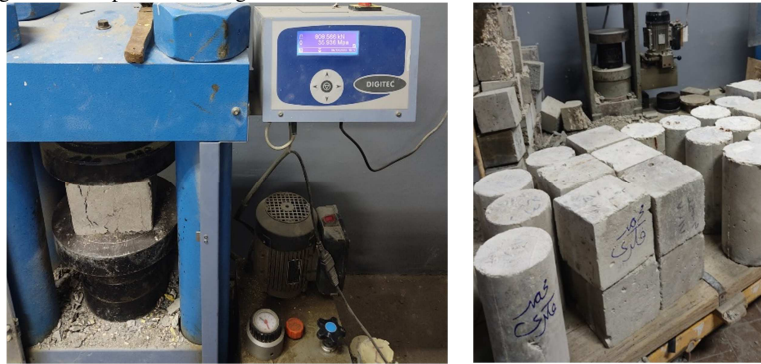
Figure 1: Testing the compressive strength of the cubes
