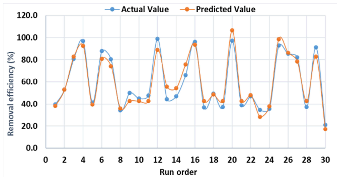
Figure 9: Diagnostic plots of the comparison between predicted and actual values of removal process of MB dye using the prepared nanocomposite.
