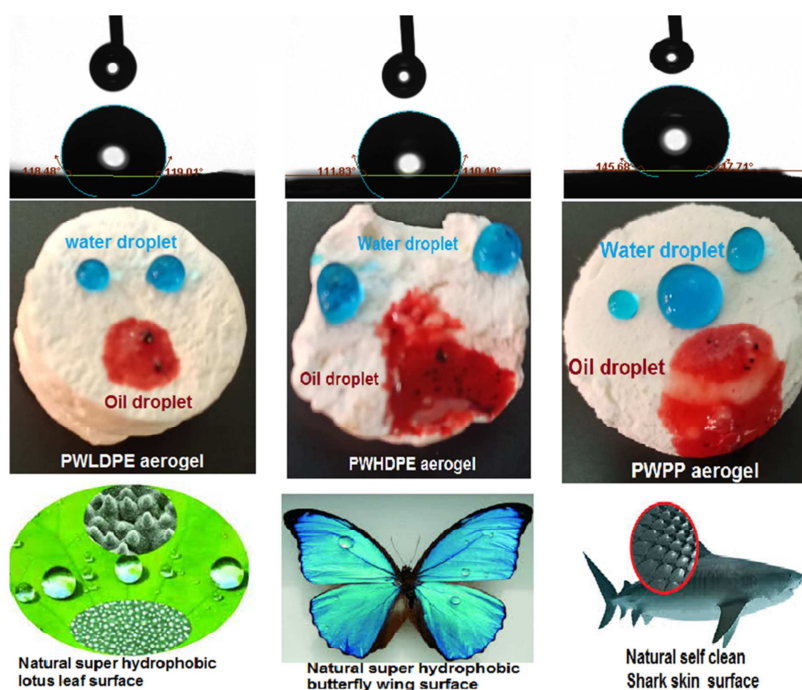
Figure 6: Wettability of the prepared PW aerogels and the natural super hydrophobic surfaces.
