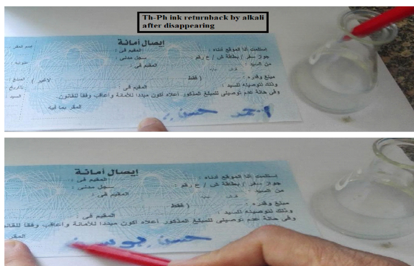
Fig. 19: Reconquest of Th-ph ink from C4 paper as an examples of papers under investigations by using 1.0 M KOH at 25°C.
