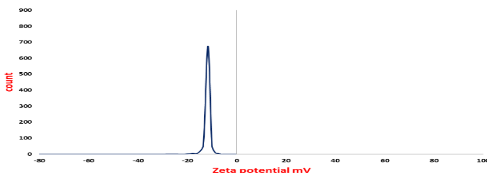
Figure 4. Zeta Potential Analysis Confirms Enhanced Stability of Nano Cadmium Complex (-15 mV).
