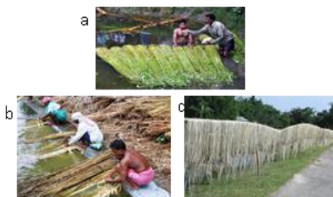
Figure 7 a) Jute water retting, (b) Jute Extraction and (c) Jute fiber drying [18]
