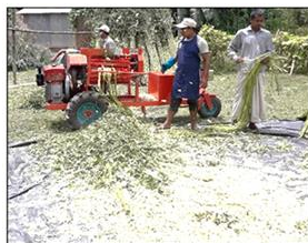
Figure 5 Jute fiber extraction by the developed Aashkol[22].
