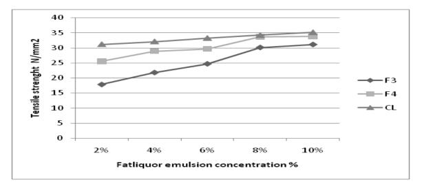
Fig. 2. Tensile strength of lubricated leather at different emulsion concentrations.
