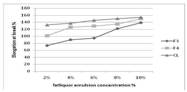
Fig. 3. Elongation at break of lubricated leather at different emulsion concentrations
