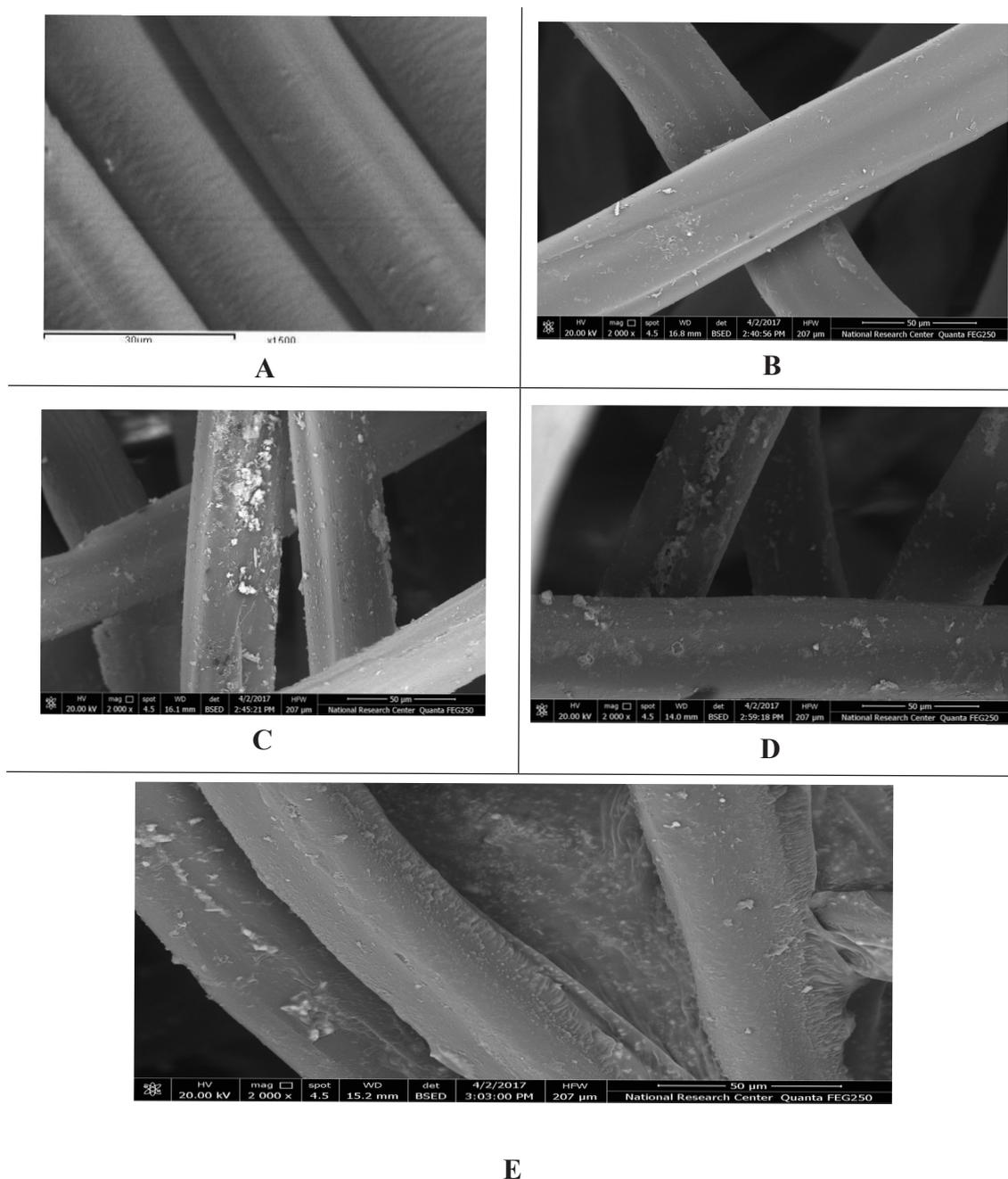
Fig. 1. SEM of blank nylon-6 nonwoven fabrics and grafted with PVQAs (2000x)
