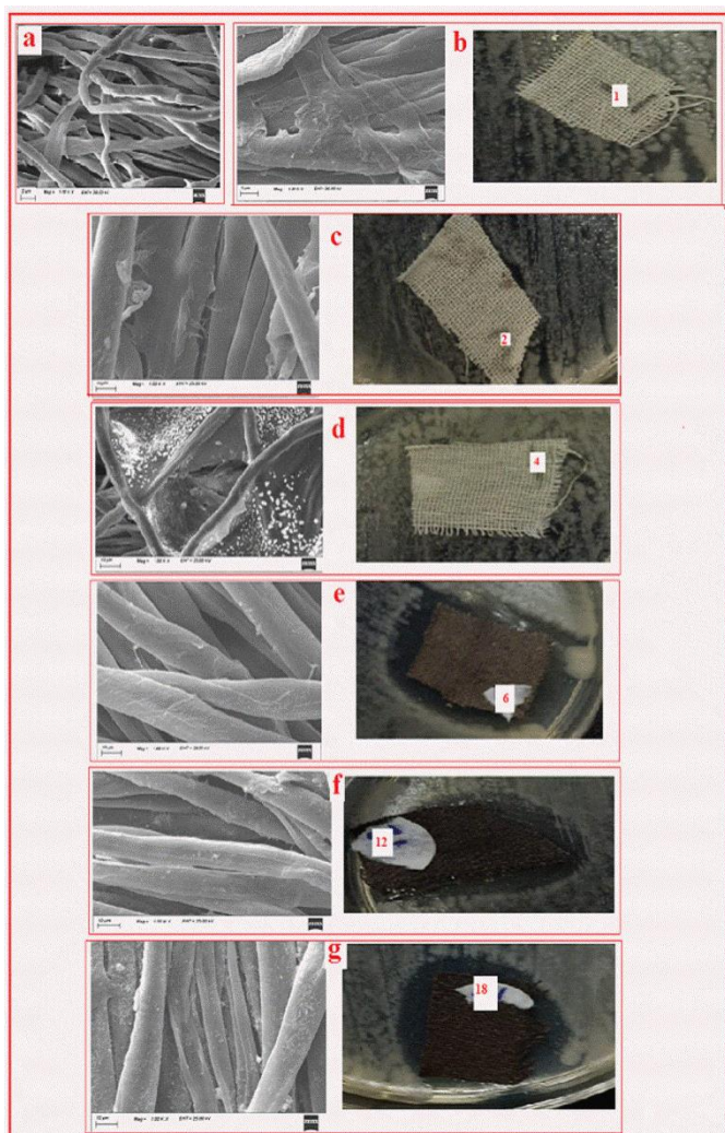
Figure 13. SEM images and dishes of cotton fabrics untreated and treated against bacteria: (A) pure cotton fabrics without bacteria, (B) fabrics by immersing in EG/CMC/PEG at 0 kGy, (C) fabrics by immersing in CMC/PEG/EG at 5 kGy, (D) fabrics by immersing in EG/CMC/PEG at 25 kGy, (E) fabrics by immersing in EG/CMC/PEG/Ag (0.006%)/ ( 12 \times 10^{-3} %) nano CuO at 5 kGy, (F) fabrics by padding in EG/CMC/PEG/Ag (0.006%)/ (1/2%) nano CuO at 25 kGy and (G) fabrics by immersing in EG/CMC/PEG/Ag (0.006%)/ (2.0%) nano CuO at 5 kGy
