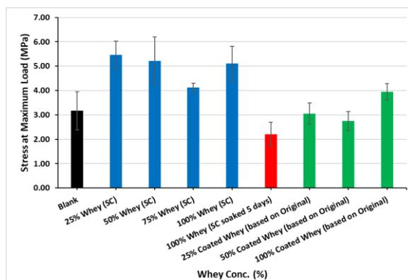
Fig3 Stress at maximum load versus whey concentration
