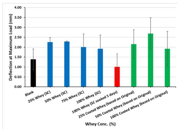
Fig2 Deflection at maximum load versus whey concentration
