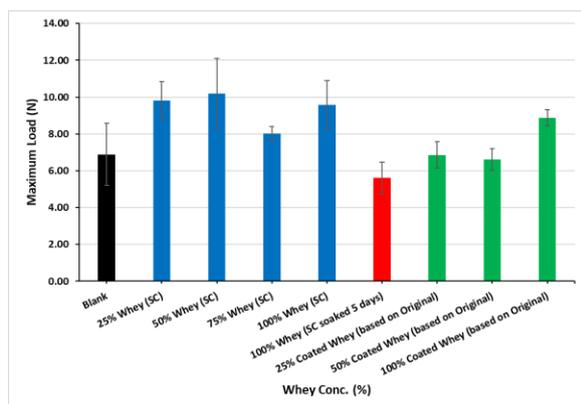
Fig1 Maximum load versus whey concentration
