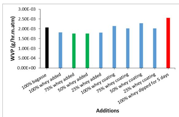
Fig 6 water vapor permeability versus whey concentration
