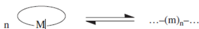
Figure 8: Ring opening of a cyclic monomer (M) and “m” is the repeating unit derived from M
