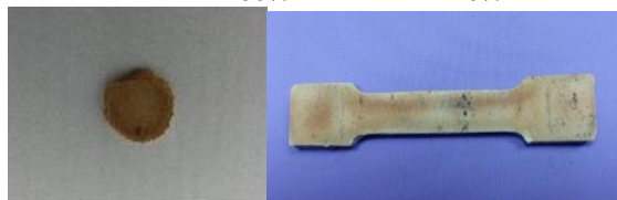
Fig. 1. Pure PBSA circle and dimple shape specimens resulted from dry mixing
