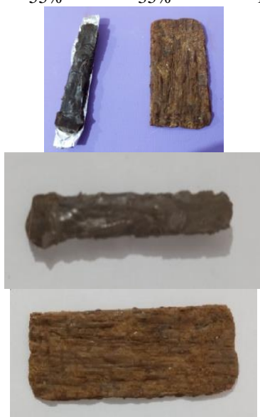
Fig. 2. PBSA /PLA / Nanoclay composites specimens resulted from melt casting
