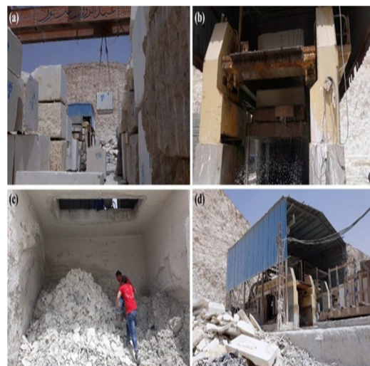
Figure 1: Ornamental stone blocks are transported from the store house to be processed (a); the blocks are cut by industrial saws (b); (“Sahala” after pressing by filter press (c) and Cuttings and shreds in the work environment (d) in Shaq Al-Teaban industrial zone.
