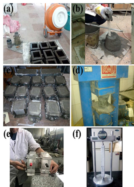
Figure (2): Concrete pan mixer and casting molds (a), slump test (b), cast concrete cubes (c), compressive strength machine (d), rapid chloride permeability testing (RCPT) (e) and alkali-aggregate reaction testing setup (f).
